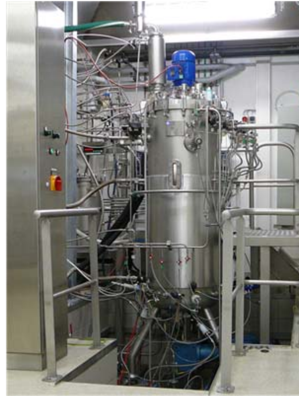
Bioreactor with 400-Liter working volume for enzyme production and SSF-process in pilot scale
