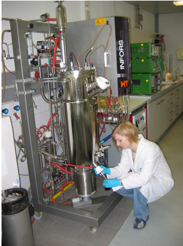
Bioreactor with 25-Liter working volume, sampling
