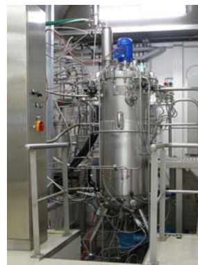
Bioreactor with 400-L working volume for enzyme production and SSF-process in pilot scale (in co-operation with UFZ-Centre for Environmental Biotechnology, UbZ).
