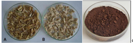
Untreated straw (A), pre-treated straw according to the NP-process (B), wheat straw-lignin resulting from the NP-process (C)
